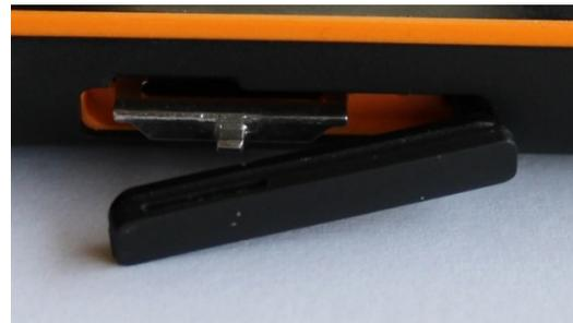
Then insert the SIM card(s) into the slot(s) with the included accessory (vividly insert the tip into the slot) and insert the card(s) holder (the picture next to this text) into the slots according to drawings and gently slide the card tray.
