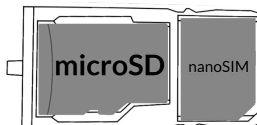
turn off the phone and, with the included accessory, open and slide out the card(s) holder. Insert the memory card into the slot according to the picture above (**instead of the nano SIM1 card**).
